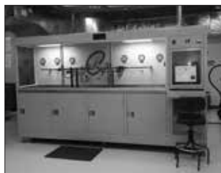
Fluid Care Center: Multi-Pass Test Stand
