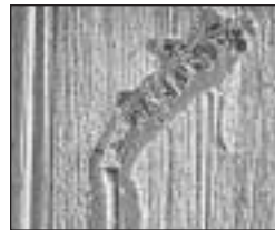
Figure 13. Contaminate embedded in the surface of a friction bearing
