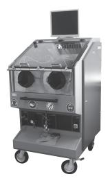
The Cleanliness Test Unit (CTU 1000) is designed to determine the technical cleanliness especially present on minor contaminated components. By determining the type, size and quantity of the contamination, quality standards can be checked and documented and the necessary steps towards optimization can be taken.
