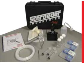
The Schroeder EasyTest Patch Kit (EPK) provides the necessary tools to determine the level of solid particulate contamination present in a fluid sample. Using the vacuum pump contained in the kit, the fluid sample is drawn through a membrane patch. The residual particulate left on the patch is viewed under a microscope and compared to photos of known contamination levels in the L-2711 Schroeder Contamination Handbook (included).
