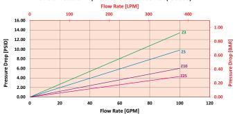
$$\triangle \mathbf{P}_{\text{filter}} = \triangle \mathbf{P}_{\text{housing}} + (\triangle \mathbf{P}_{\text{element}} * \forall_f)$$
