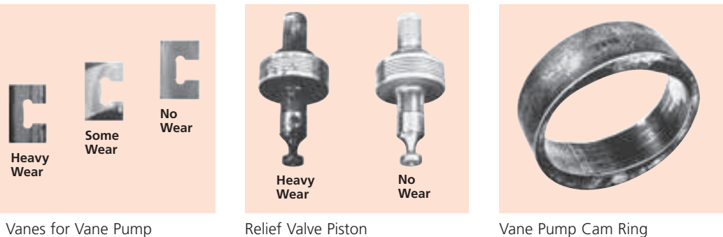
Figure 1. Typical Examples of Wear Due to Contamination
