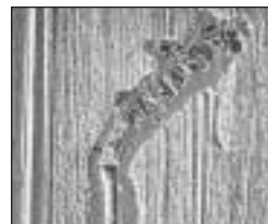
Figure 13. Contaminant embedded in the surface of a friction bearing
