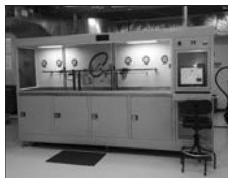
Fluid Care Center: Multi-Pass Test Stand
