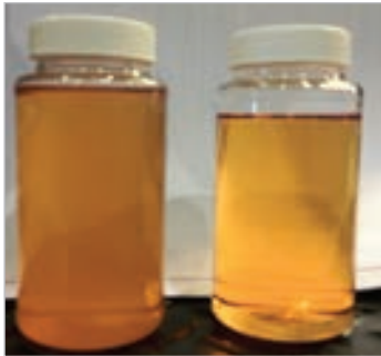
BDC: 25 gpm Fuel Filter/Coalescing Cart 25,000 ppm became 250 ppm - water only
