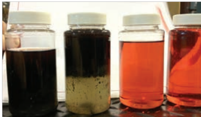
Example: BDC Single Pass Results - Diesel Storage Tank Bottom
