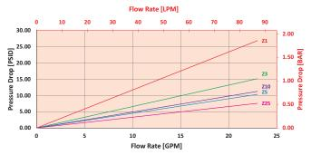
5TBZ Element Pressure Drop versus Flow Rate at 32 cSt (150 SUS)
