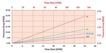
$$\Delta P_{filter} = \Delta P_{housing} + (\Delta P_{element} *V_f)$$
