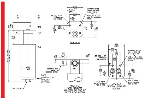
Metric dimensions in (). Dimensions shown are inches (millimeters) for general information and overall envelope size only. For complete dimensions please contact Schroeder Industries to request a certified print.
