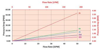
$$\triangle P_{\text{filter}} = \triangle P_{\text{housing}} + (\triangle P_{\text{element}} * \mathbf{v}_f)$$
