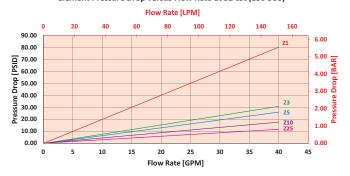
9HZ Element Pressure Drop versus Flow Rate at 32 cSt (150 SUS)
