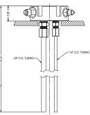
Reservoir Mounting Pattern: Fits standard 6-bolt Supply Port Thread Size: 9/16-18 UN Return Port Thread Size: 7/16-20 UN Breather Port Thread Size: 3/4" NPT
