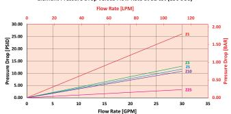
$$\triangle \mathbf{P}_{\text{filter}} = \triangle \mathbf{P}_{\text{housing}} + (\triangle \mathbf{P}_{\text{element}} * \forall_f)$$
