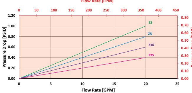
$$\Delta P_{\text{filter}} = \Delta P_{\text{housing}} + (\Delta P_{\text{element}} * v_f)$$
