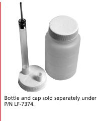
The Probalizer Sampling Test Point provides a point of access for obtaining representative fluid samples from an operational hydraulic system. The downstream channel is specially sized to accept the sampling probe from a customized cap/probe assembly screwed onto a sample bottle. (See photo). Use of this system minimizes leakage and helps to maintain the integrity of the sample.
