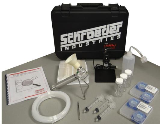
The Schroeder EasyTest Patch Kit (EPK) provides the necessary tools to determine the level of solid particulate contamination present in a fluid sample. Using the vacuum pump contained in the kit, the fluid sample is drawn through a membrane patch. The residual particulate left on the patch is viewed under a microscope and compared to photos of known contamination levels in the L-2711 Schroeder Contamination Handbook (included).
