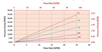
$\triangle P_{\text{filter}} = \triangle P_{\text{housing}} + (\triangle P_{\text{element}} * V_f)$
